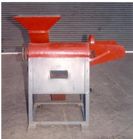
Fig. 2: Maize sheller (Power operated).
